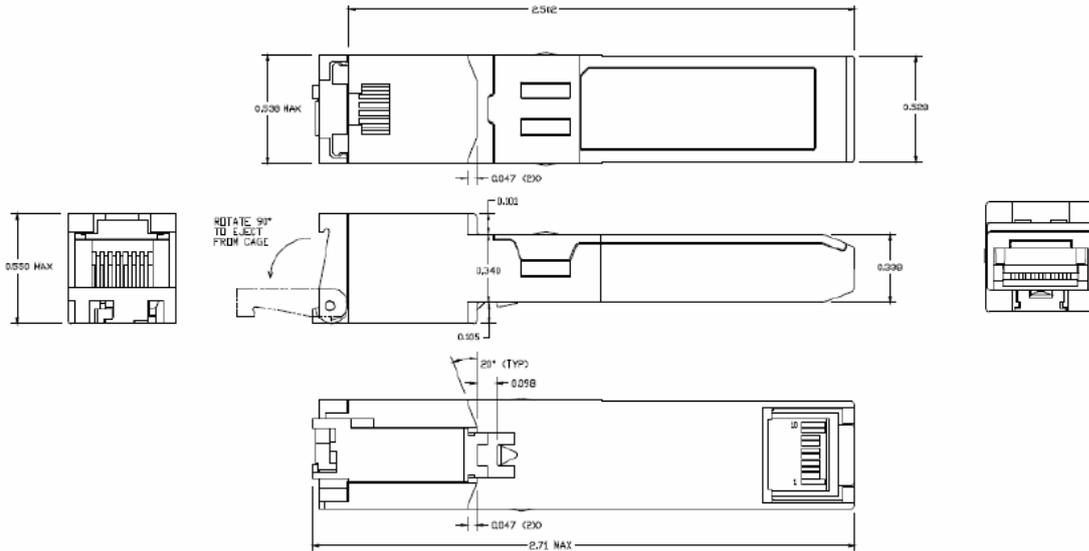
**Figure 2. XSUEx1-M1RN mechanical dimensions**
