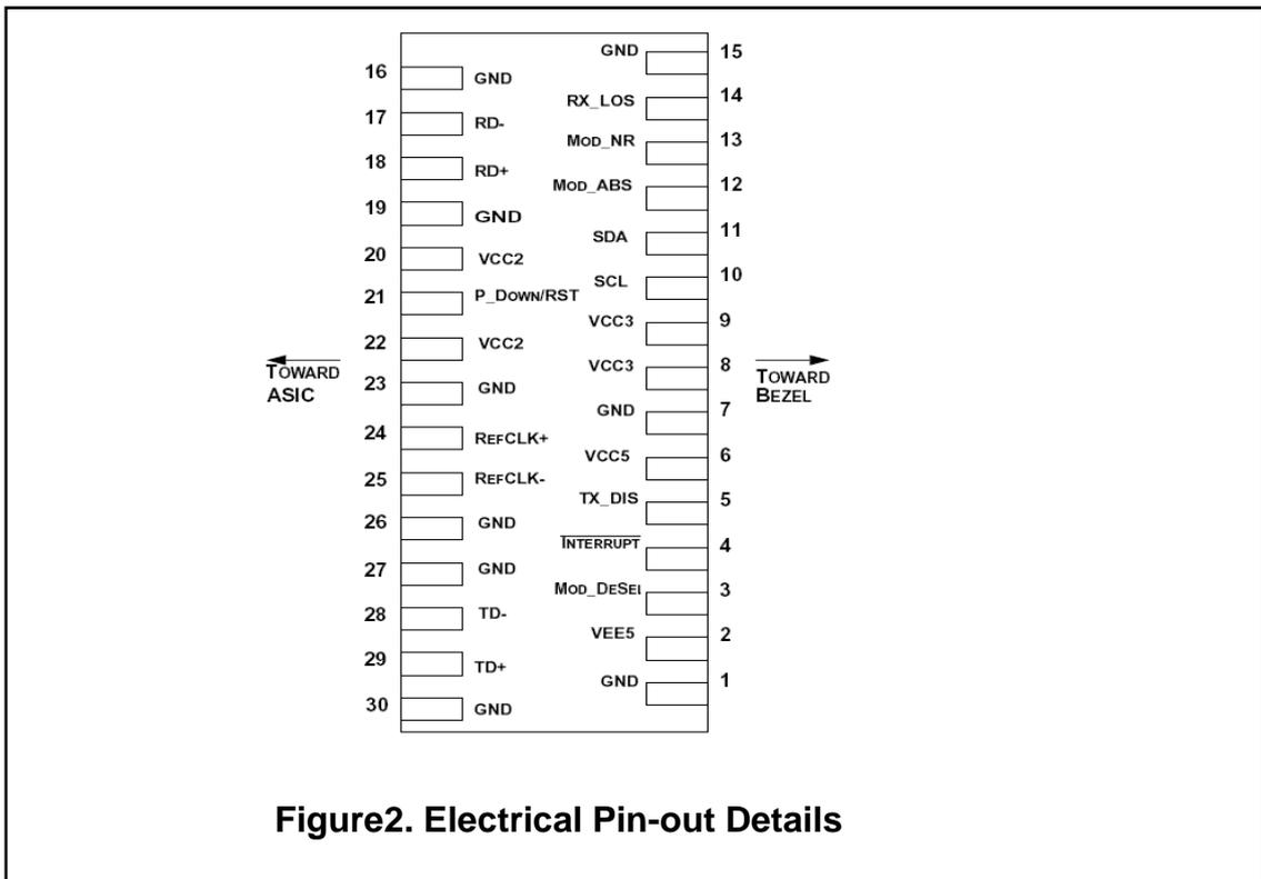
Figure2. Electrical Pin-out Details
